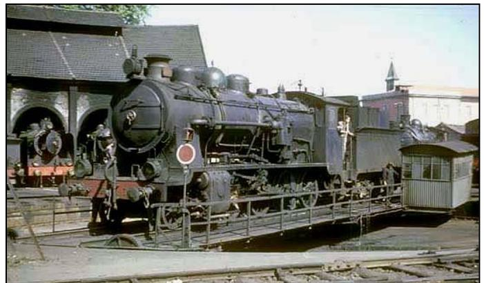
The photos above were taken by John Champion at Campanhã locomotive shed in May 1964. They show (left) NBL design 2-8-0 compound No. 762 (one of the Schwartzkopff engines) running light in the yard and (right) Former Sul e Sueste 2-8-0 number No 713 built by North British (22709/1921) on the turntable.
