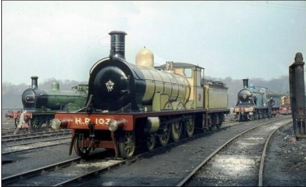
The Highland Railway 'Jones Goods' locomotives were notable as the first engines in the UK with the 4-6-0 wheel arrangement. 15 were built by Sharp Stewart in 1894 and one, No 103 has survived into preservation.
